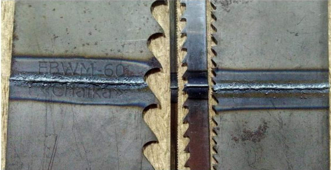
Flash Butt Welding
